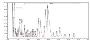
Figure 2. HPLC-RI chromatogram of palm pressed fiber oil (PPFo) extracted via cold extraction
